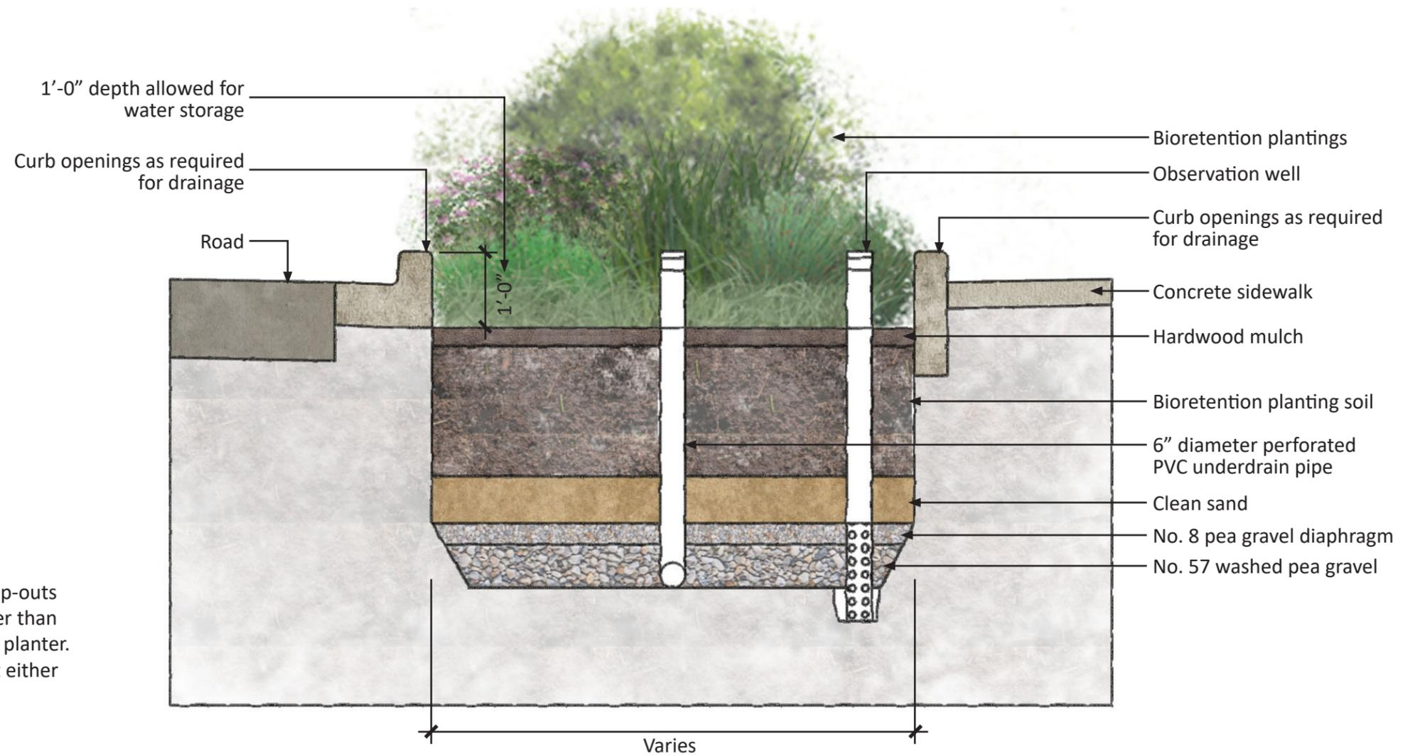
**Figure 1. Bioretention Planter Typical Section.**
