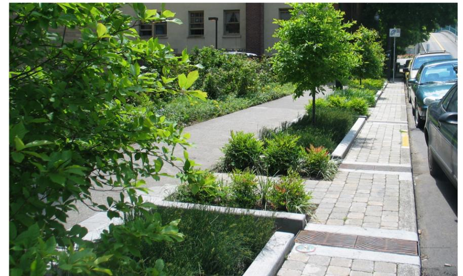
Image of a stormwater planter. Courtesy of Jersey Water Works.
